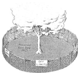
Tree fencing shall consist of 4' high minimum orange polyethylene laminar safety netting.
